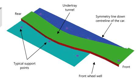
FEA model of the carbon fibre undertray.
