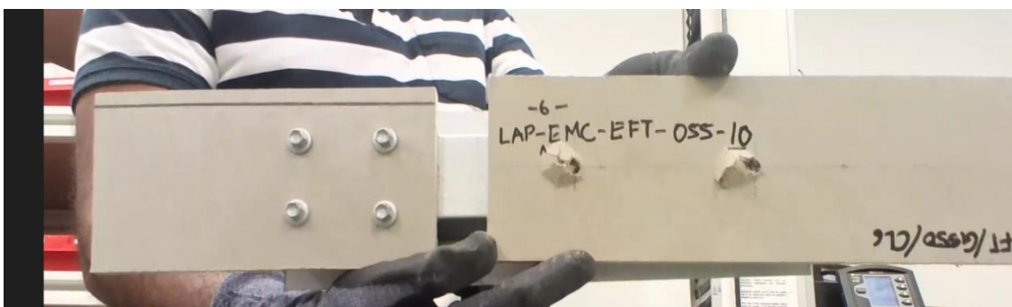
Figure 3: Lap Shear Test Specimen after Screw Bearing Failure
